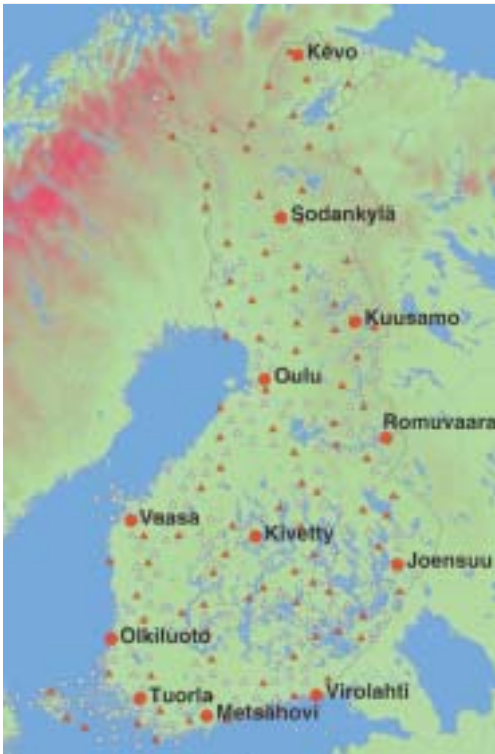
Figure 2. FinnRef, the Finnish permanent GPS network maintained by the Finnish Geodetic Institute (roundels), the national EUREF-FIN coordinate system (red triangles), and the triangulation network, I order (yellow triangles).
